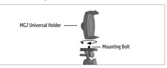
2 Insert device and adjust as needed.
